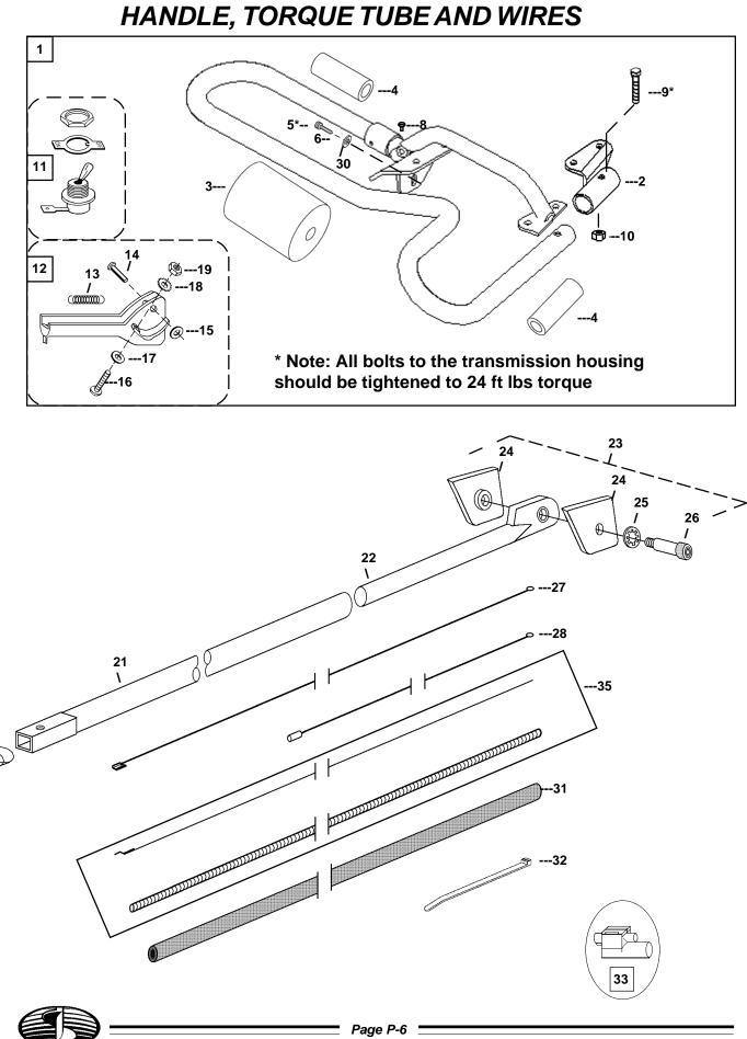
HANDLE, TORQUE TUBE AND WIRES
